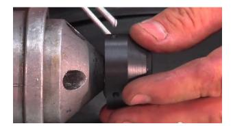
2. Slide cylinder head saver over spring compressor foot and insert retainer clip.
