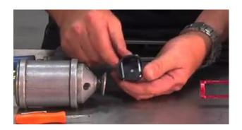
1. To attach cylinder head saver to valve spring compressor remove steel U-shaped retainer clip.
